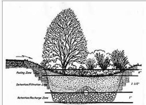
Cross-section of a typical rain garden
